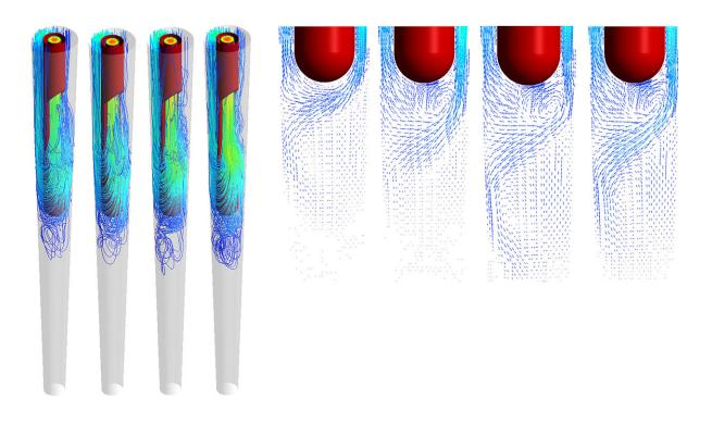
Left: Streamlines of the irrigation fluid; right: Velocity vectors at the recirculation zone next to the needle tip. Credit: Hanhui Jin
