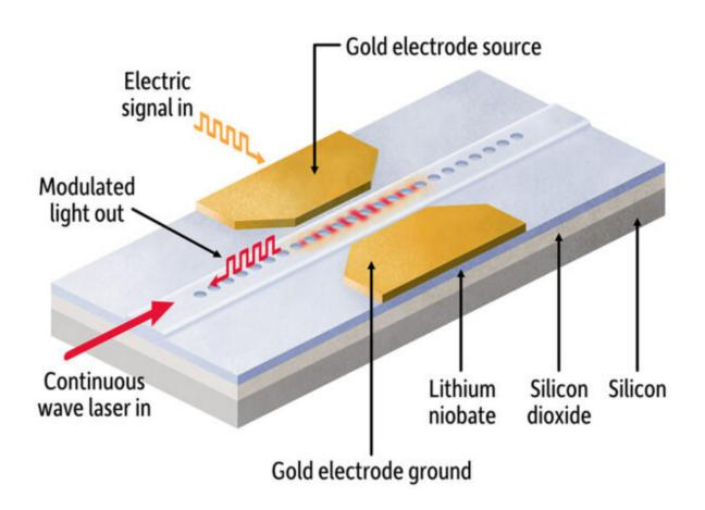
A schematic drawing shows an electro-optical modulator developed in the lab of Qiang Lin, professor of electrical and computer engineering. The smallest such component yet developed, it takes advantage of lithium niobate, a "workhorse" material used by researchers to create advanced photonics integrated circuits. Credit: University of Rochester illustration / Michael Osadciw
