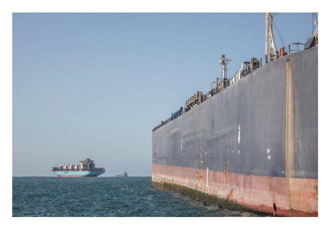
Since 2016, ship-to-ship refuelling, or bunkering, has been possible in Algoa Bay—the main storage tanker can hold 100,000 metric tons of fuel
