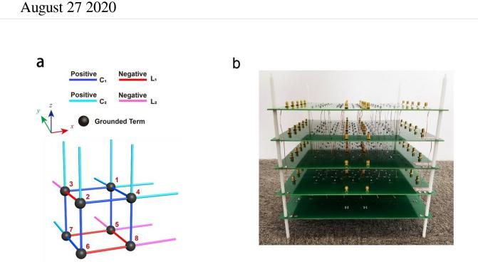
(a) Theoretical mode of the unit cell. (b) Fabricated sample which contains 2.5×2.5×2.5 unit cells. Credit: by Shuo Liu, Shaojie Ma, Qian Zhang, Lei Zhang, Cheng Yang, Oubo You, Wenlong Gao, Yuanjiang Xiang, Tie Jun Cui & Shuang Zhang
