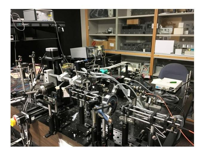
Researchers have developed a unique synchronized high-speed OCT/scanning light ophthalmoscope (SLO) system that captures the function of the retina's rods and cones. The OCT images are co-registered with SLO images to pinpoint the location and type of photoreceptors captured in the series of 3D OCT images. The optical setup is shown. Credit: Mehdi Azimipour, UC Davis Eye Center.
