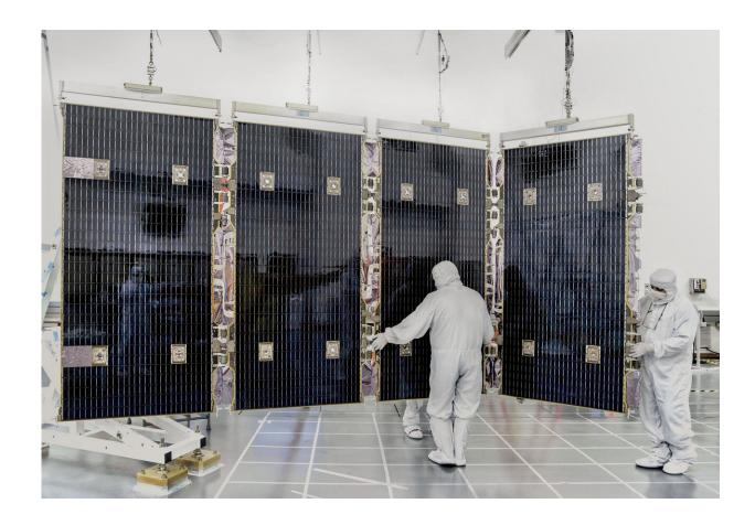
Technologists holding the solar array of the James Webb Space Telescope after a test of the array earlier in 2020. The fifth panel of the solar array is folded behind the fourth in this image. Credit: NASA/Chris Gunn
