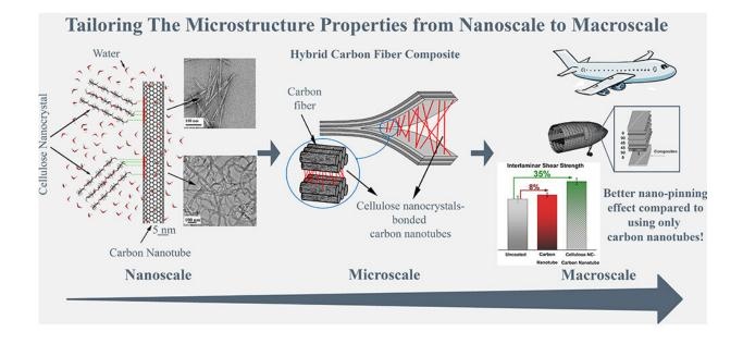
Schematic showing how cellular nanocrystals help in evenly distributing carbon nanotubes on the carbon-fiber composites. Credit: Dr. Amir Asadi/Texas A&M University College of Engineering
