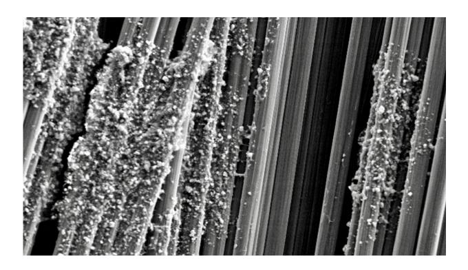
Electron micrograph of cellular nanocrystals on the carbon fibers. Credit: Dr. Amir Asadi/Texas A&M University College of Engineering
