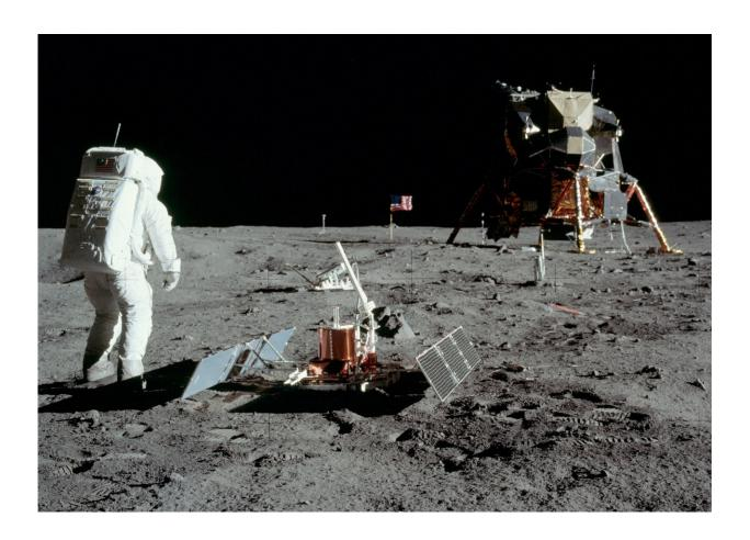
The first seismometer on the moon, with solar panels and an antenna pointed at Earth, was placed there by Apollo 11 astronauts and tested by Buzz Aldrin stamping his foot. Credit: NASA
