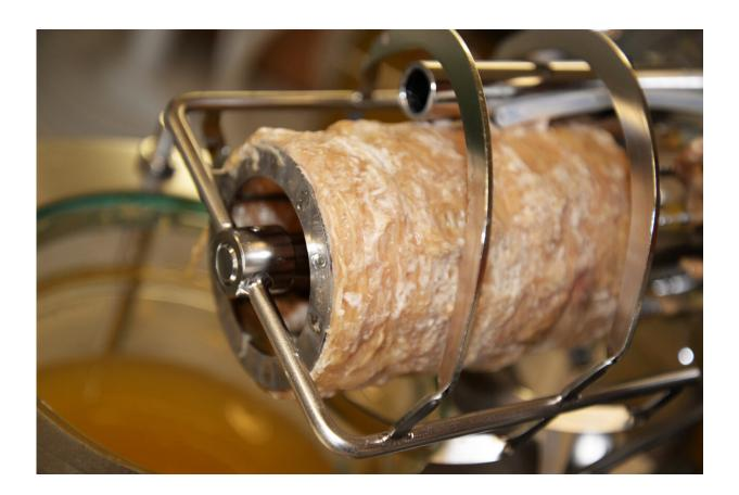
Fungal biofilm growing on an oxygen permeable, helically coiled tubular membrane in an otherwise anaerobic bioreactor. The biofilm is removed from the reactor at the end of a fermentation run. Credit: M. Studer (BFH)
