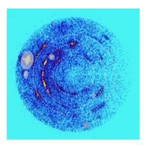
X-ray diffraction images showing the new form of silica created by sending an intense shock wave through a sample of quartz using a specialized gas gun. When the x-rays bounce off repeating planes of a crystalline structure, they scatter. This creates a distinctive ring pattern. Each ring is associated with a different plane and together this data can tell researchers about the material's atomic-level architecture. Credit: Sally June Tracy, Stefan Turneaure, and Thomas Duffy.
