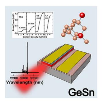
Schematic illustration of electrically injected germanium-tin laser and its power output versus current and spectrum characteristics. Credit: University of Arkansas
