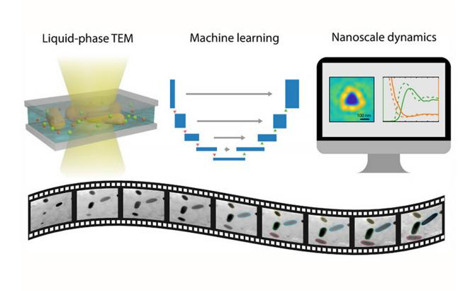
The schematic shows a simplified version of the steps taken by researchers to connect liquid-phase electron microscopy and machine learning to produce a streamlined data output that is less tedious to process than past methods. Credit: ACS and the Qian Chen group
