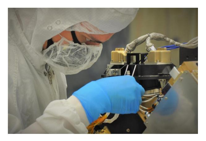
A Lucy team member installs the scan mirror on the L'Ralph Instrument at Goddard Space Flight Center in preparation for integration into the spacecraft. The SwRI-led mission just passed a major milestone. Credit: NASA/GSFC
