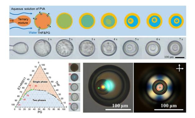
Liquid crystal particles with multiple layers formed through phase separation process developed by KIST-KAIST joint research team. Credit: Korea Institue of Science and Technology(KIST)
