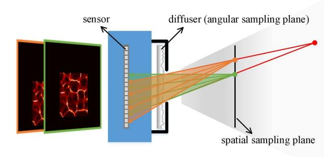
A diffuser is placed at a small distance in front of a sensor so that a temporally incoherent point source in the detectable field-of-view generates a high-contrast pseudorandom pattern. The elementary sub-beams, represented by their center light rays, are angularly encoded in the pattern Credit: Zewei Cai, Jiawei Chen, Giancarlo Pedrini, Wolfgang Osten, Xiaoli Liu, and Xiang Peng
