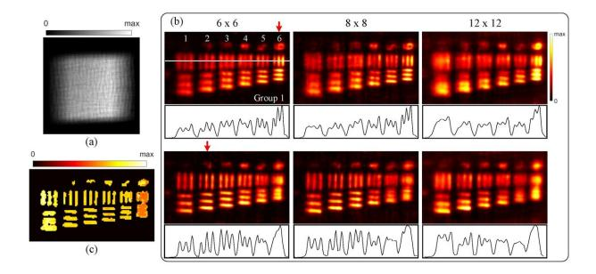
a, A raw image was captured by the system. b, Light fields in different spatioangular samplings were reconstructed from the captured image. Respective focal stacks were then obtained from these reconstructed light fields by performing digital refocusing. c, By using the focal stack, the depth of the measured object was estimated Credit: Zewei Cai, Jiawei Chen, Giancarlo Pedrini, Wolfgang Osten, Xiaoli Liu, and Xiang Peng
