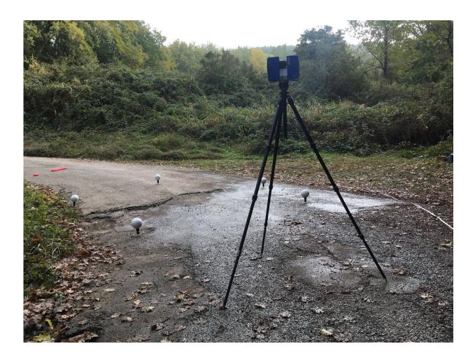
A field survey measured the ground displacement along the surface rupture. The photograph shows a laser scanner used to measure ruptures and fissures. This method, together with InSAR data, identifies localised deformation right on the fault (~45%) and deformation distributed off-fault (~55%). Credit: © Jean-François RITZ / Géosciences Montpellier / CNRS Photothèque
