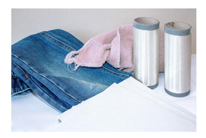
Wound onto a spool, the viscose filament yarn was spun from recycled cotton provided in form of cellulose sheets. Researchers at the Fraunhofer IAP have found a way to turn cotton clothes such as jeans into new high-quality garments rather than lowly cleaning rags. Credit: Fraunhofer IAP
