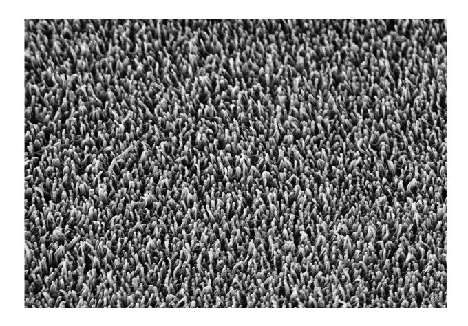
The nanopillars on the surface of a dragonfly wing (magnified 20,000 times). Credit: RMIT University
