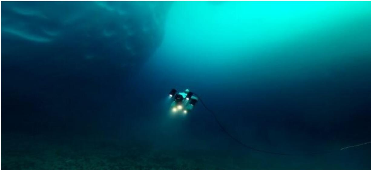
A remote operated vehicle (ROV) moves through the water collecting samples.
