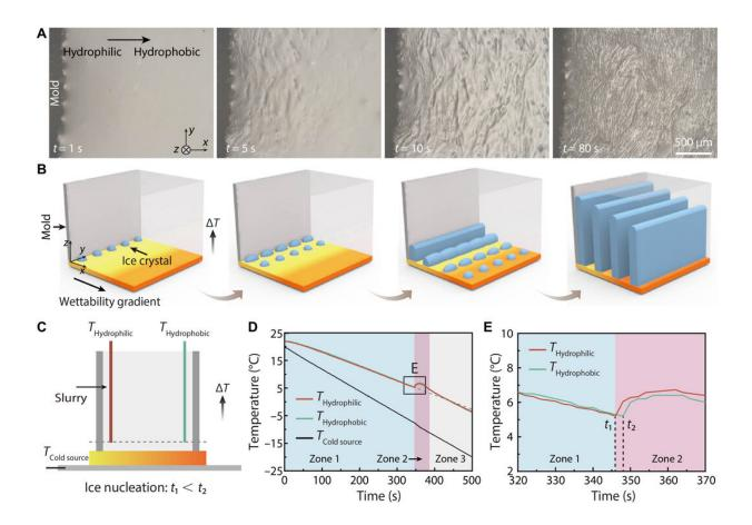
Observation of the freezing process. (A) Top-view optical images showing successive nucleation of ice crystals from the hydrophilic to hydrophobic region
