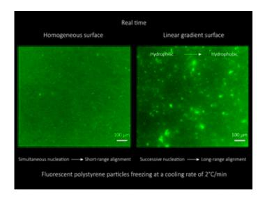
Observing the freezing process across a homogenous surface vs. a linear gradient surface. Credit: Science Advances, doi: 10.1126/sciadv.abb4712
