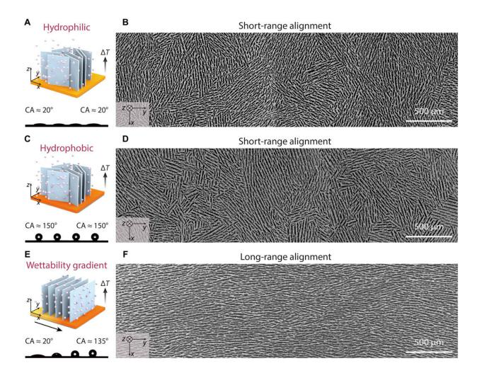
Freeze-casting technique using copper surfaces with different wettability and the resulting scaffolds. SEM images were taken from the cross section of 1-cm height parallel to the cold surface. (A to D) When freezing on the
