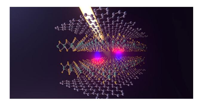
Schematic illustration of the electron-hole pairs (electron: pink, hole: blue), which are formed by absorption of light in the two-layer molybdenum disulfide layer. Credit: Nadine Leisgang and Lorenzo Ceccarelli, Department of Physics, University of Basel
