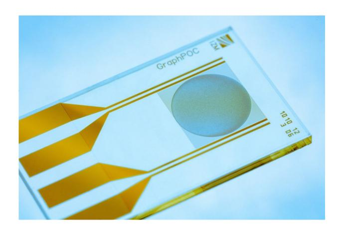
Fraunhofer researchers are developing graphene oxide-based biosensors to detect bacterial and viral infections within just 15 minutes. Credit: Fraunhofer IZM
