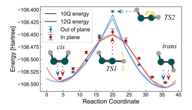
Energy predictions of molecular geometries by the Hartree-Fock model simulated on 10 qubits of the Sycamore processor. Credit: Google
