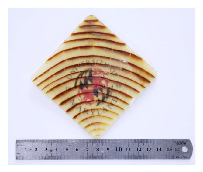
By removing a key component of wood, a block of wood can be made transparent, with natural abilities to block heat and direct light, researchers at the University of Maryland showed. Credit: A. James Clark School of Engineering, University of Maryland
