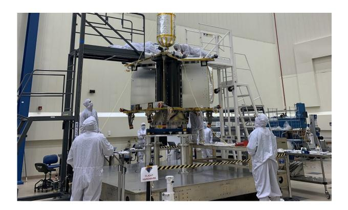
Engineers install Lucy's oxidizer tank into the spacecraft structure in the High Bay at Lockheed Martin. The SwRI-led mission has entered the final stage of development be-fore the spacecraft is scheduled to launch in 2021. Credit: Lockheed Martin
