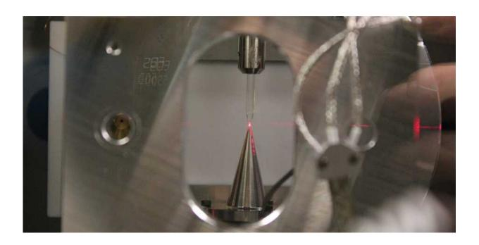
The scientists inject water from above into the analysis chamber, where it forms a short microjet that meets a laser beam. Credit: ETH Zurich / Inga Jordan
