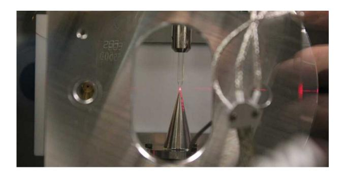
The scientists inject water from above into the analysis chamber, where it forms a short microjet that meets a laser beam. Credit: ETH Zurich / Inga Jordan
