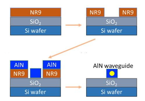
Schematic showing the steps for creating the optical waveguide. Credit: Texas A&M University College of Engineering
