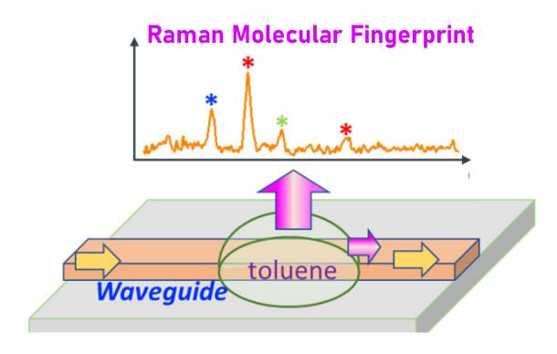
Aluminum nitride optical waveguide carries the laser beam to a test sample. Scattered light reveals the sample's Raman molecular fingerprint. Credit: Texas A&M University College of Engineering
