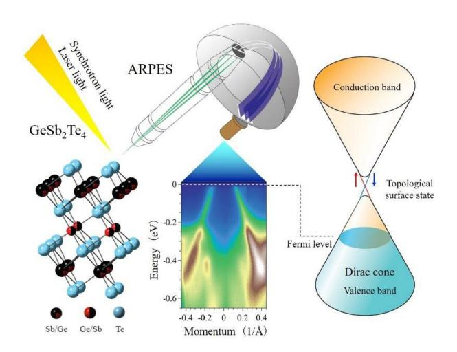
(Left) Crystal structure for the intermixed crystalline phase of the phase-change compound GeSb2Te4. (Middle) Angle-resolved photoemission spectrum of crystalline GeSb2Te4 by showing the linearly dispersive band crossing the Fermi level. (Right) Schematic band structure of the crystalline GeSb2Te4 based on
