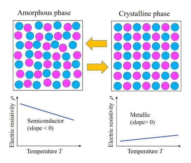
Schematic for the amorphous phase (left) and crystalline phase (right) of the phase-change materials which demonstrate the atomic rearrangement during the phase transition. The amorphous phase shows a semiconducting behavior with a large electrical resistivity while the crystalline phase behaves metallic with a much lower electrical resistivity. Credit: Akio Kimura, Hiroshima University
