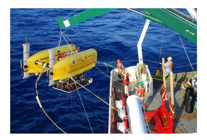
The hybrid remotely-operated vehicle Nereus was used to collect seafloor samples, in addition to remotely operated vehicle Jason II, at Piccard vents at Mid-Cayman Rise. Credit: Jill McDermott
