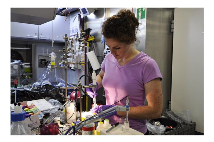
Lead author Jill McDermott performing a chemical analysis called titration to analyze the hydrogen sulfide content of vent fluid samples onboard the R/V Falkor in 2013. Credit: Julie Huber
