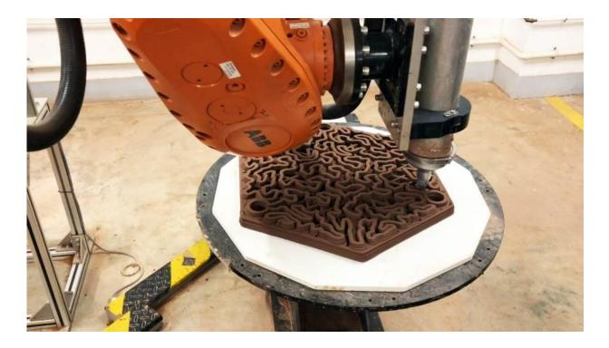
A 3-D-designed reef tile was printed through a robotic 3-D clay printing method with generic terracotta clay and then fired at 1125 degrees Celsius. Credit: Christian J. Lange
