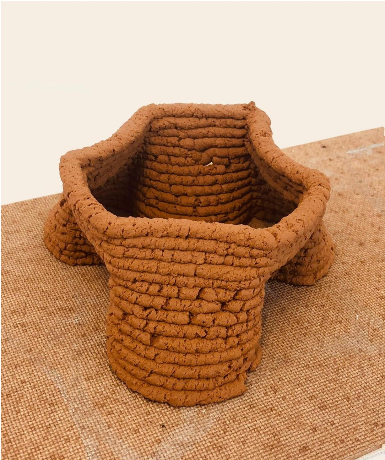
Scientists have developed a method to 3D print structures using local soil. Credit: Aayushi Bajpayee
