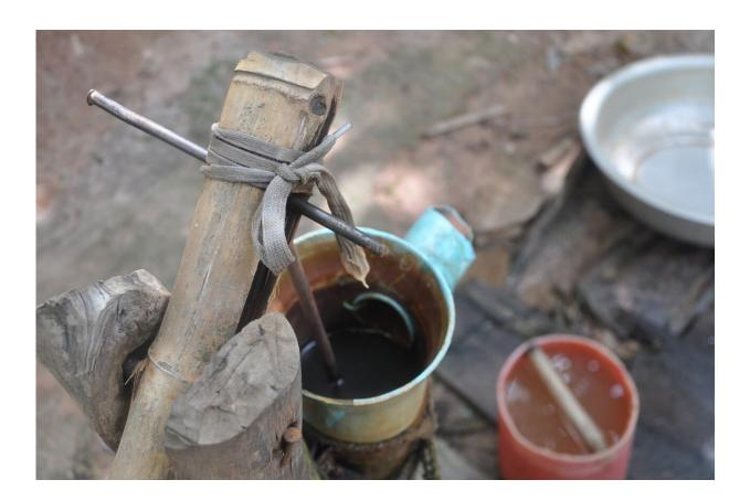
Homemade water pump in Cambodia made of PVC and bamboo. Credit: (Samantha Ying/UCR)
