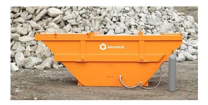
Neustark's pilot plant turns broken concrete and  $CO_2$  into stone granulate that can serve as a replacement for sand and gravel in fresh concrete. Credit: Micha Riechsteiner
