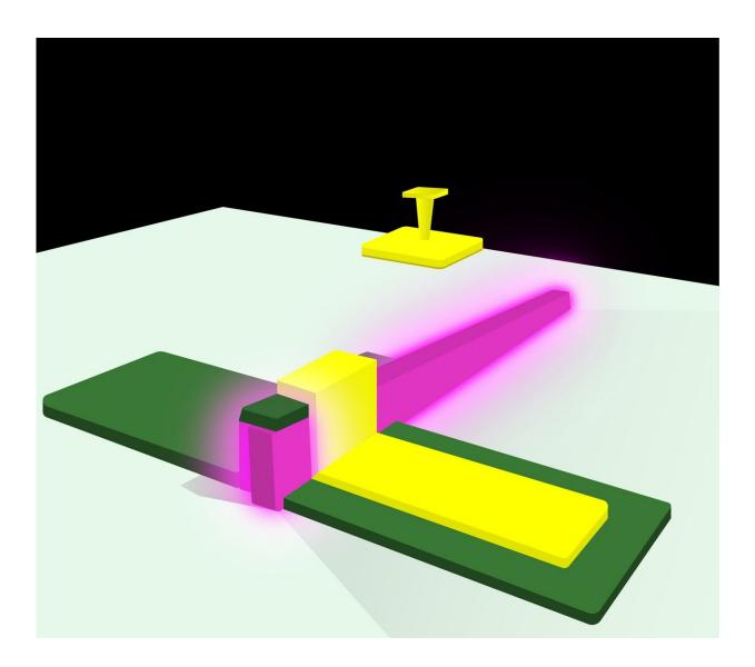
The fin LED pixel design includes the glowing zinc oxide fin (purple), isolating dielectric material (green), and metal contact (yellow atop green). Credit: B. Nikoobakht / N. Hanacek, NIST
