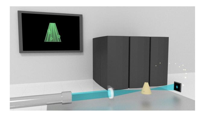
This illustration shows a coherent X-ray beam focused on a large-scale specimen while recording far-field diffraction patterns as the specimen is scanned and rotated. In the background is a computing system using automatic differentiation approaches to reconstruct a 3D image. Credit: Ming Du / Argonne National Laboratory
