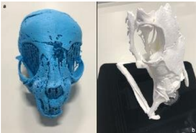
3D-prints from segmented X-ray micro tomography data. a cat mummy, b snake mummy. Credit: Swansea University
