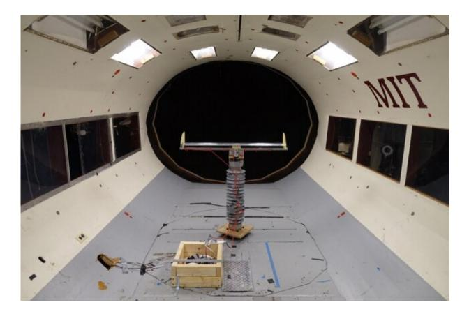
MIT researchers test the effects of a corona discharge on an electrically ungrounded model of an airplane wing inside MIT's Wright Brothers Wind Tunnel. Credit: Massachusetts Institute of Technology
