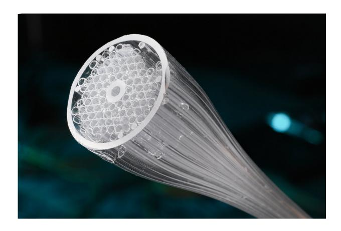
New hollow-core optical fibers that are filled with either air or gas. Credit: Alain Herzog/2020 EPFL
