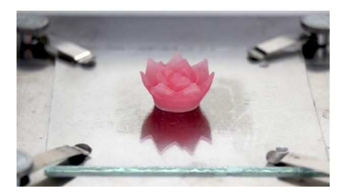
To demonstrate that fine aerogel structures can be produced in 3D printing, the researchers printed a lotus flower made of aerogel. Credit: Empa
