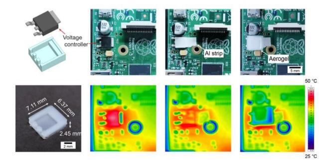
A tiny, custom-made shield made of aerogel can effectively shield heat from electronic components. These thermal images show how the heat of a voltage controller on a motherboard is shielded (left without insulation, in the middle with an aluminum strip, right with a 3D-printed, custom-made aerogel block (far left); red/violet: high temperatures; green/blue: low temperatures). Credit: Empa
