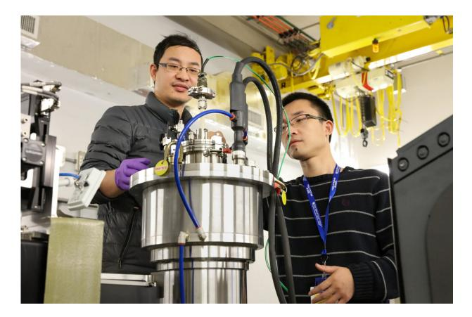
WVU researchers make adjustments to the furnace used to study high-entropy oxides under a range of temperatures from room temperature to 1,200°C (2,192°F), allowing them to better understand how HEOs form during the manufacturing process. Credit: ORNL/Genevieve Martin
