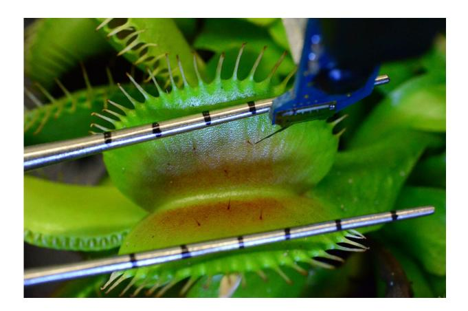
The force sensor of the microrobotic system deflects a sensory hair of a fllytrap that is kept open by the sensors of the load cell. Credit: Hannes Vogler, UZH
