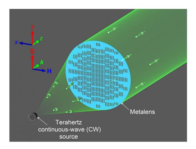
Terahertz metasurface ultra-thin collimator for power enhancement Credit: Takehito Suzuki, TUAT
