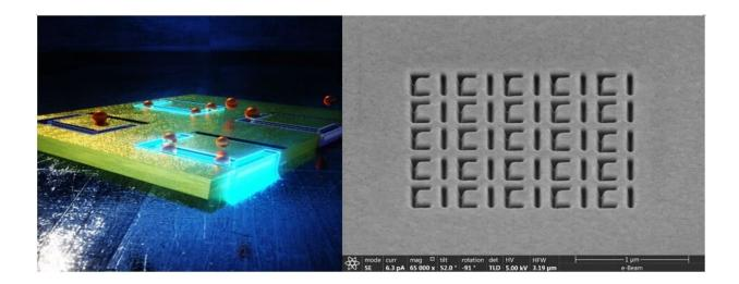
The asymmetric split rings successfully trapped 20 nm polystyrene particles at
