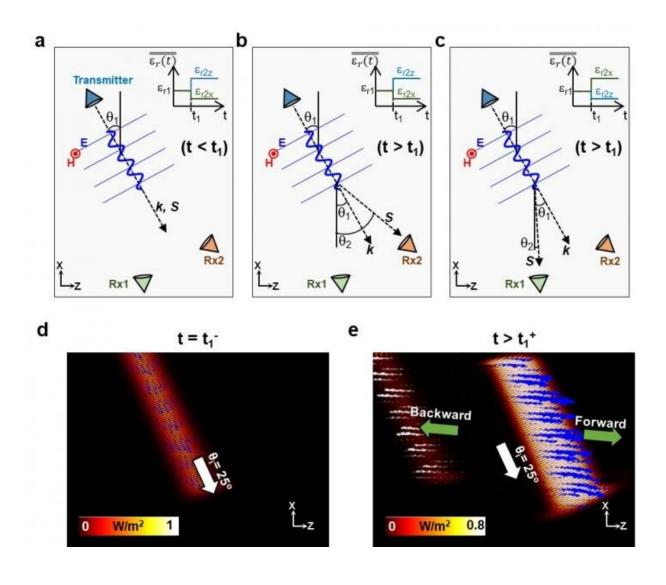
a, an incoming electromagnetic wave travels in an unbounded medium with an isotropic permittivity. b, by rapidly changing the permittivity of the medium in time from isotropic to an anisotropic tensor (with the x component of
