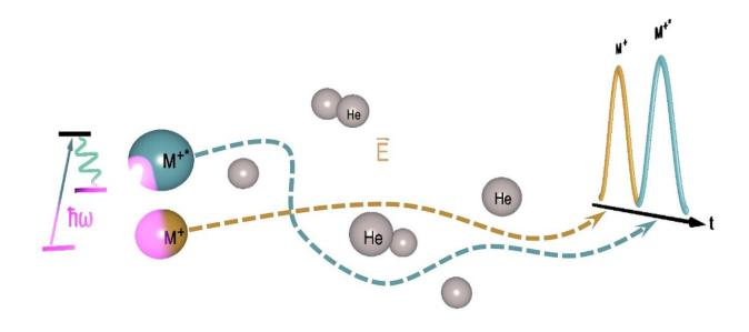
Laser resonance chromatography is based on optical excitations of ions and subsequent detection of their arrival at the detector. Credit: Mustapha Laatiaoui
