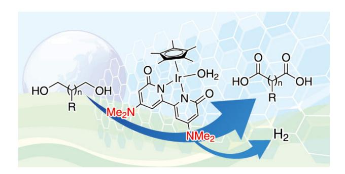
Using an iridium catalyst bound to a bipyridonate ligand, researchers were able to synthesize dicarboxylic acids from aqueous diols, with the added benefit of generating hydrogen as a byproduct. Credit: Kyoto University
