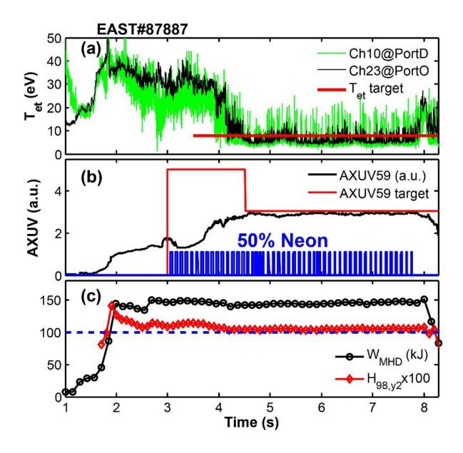
Fig.2. EAST steady-state grassy-ELM H-mode and radiative divertor compatibility operation discharge. Credit: EAST Team
