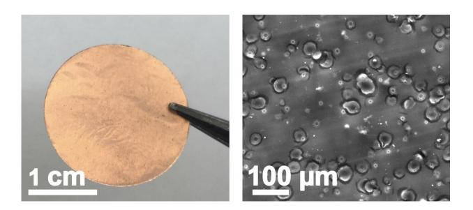
At left, a copper current collector with a laser-induced silicon oxide coating created at Rice University. At right, a scanning electron microscope image of the coating created by lasing adhesive tape on the copper collector. Credit: Tour Group/Rice University
