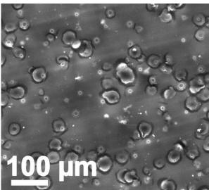
At left, a copper current collector with a laser-induced silicon oxide coating created at Rice University. At right, a scanning electron microscope image of the coating created by lasing adhesive tape on the copper collector. Credit: Tour Group/Rice University
