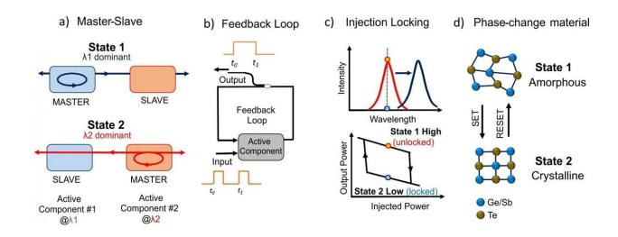
a master-slave scheme, b feedback loop scheme, c injection-locking technique and d phase-change material (PCM) properties in the case of GST compounds. Credit: by Alexoudi, T., Kanellos, G.T. & Pleros, N.
