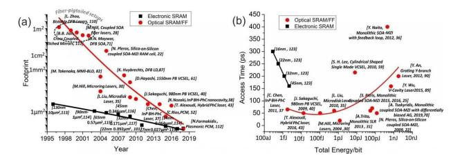
a Evolution of optical and electrical memory components in terms of footprint over the last two decades. b Memory access times in picoseconds versus total energy consumption per bit for both optical and electronic technologyin terms over the last two decades. Credit: Alexoudi, T., Kanellos, G.T. & Pleros, N.
