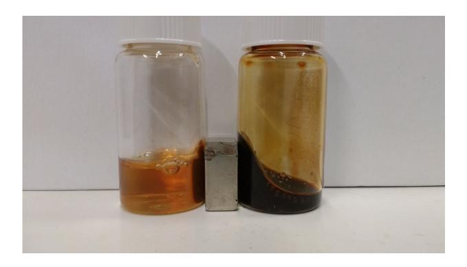
Two magnetic fluids with a magnet in the middle. Left: a non-stable magnetic fluid, where the magnetic particles in the fluid are drawn towards the magnet. Right: a fluid that does remain stable in a magnetic field. Credit: *Journal of Physical Chemistry Letters*. 2020 American Chemical Society
